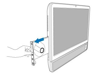
3. With the label side facing forward, place the disc in the center of the disc tray.
